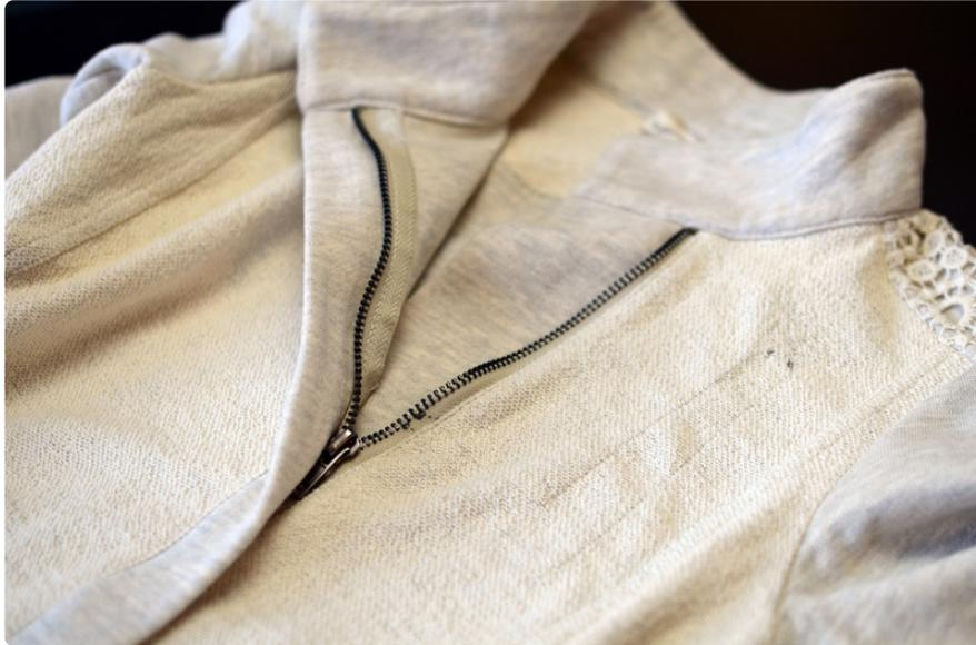
The switch works like a momentary pushbutton. As the zipper pull travels along the teeth, two pads of conductive thread are bridged, momentarily creating an electrical connection.
