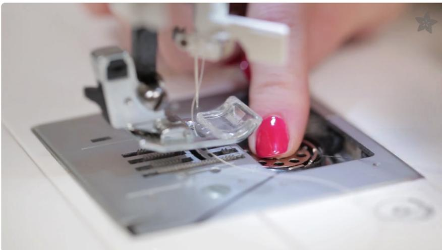
You can put 2-ply thread in the bobbin of your sewing machine, then pick up long tails with a needle and hand-stitch the rest.
