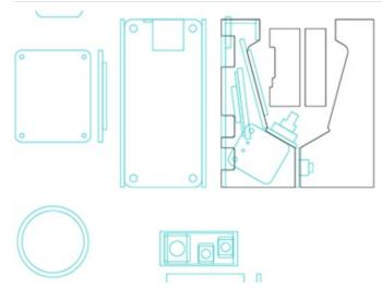
Using calipers, I measured each part and came up with a case idea. Rather than fully enclose everything, some elements (the Perma-Proto board holding the controls, plus the Raspberry Pi Zero board itself) would themselves become *elements* of the structure.
