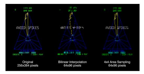
This software-based scaling isn't the most optimal route...I'm *certain* Dispmanx could handle it on the GPU using a 2-stage bilinear scale with an intermediate canvas of some sort...but nanoscreen was just an evening project and I couldn't get into that depth of understanding with Dispmanx; software scaling was familiar and comparatively easy, and
