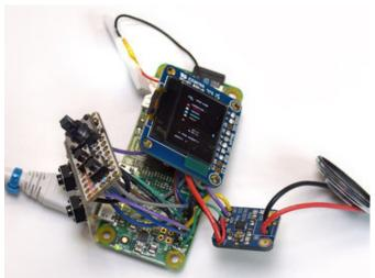
Before enclosing everything, a dry run is imperative! I'd already set up the software (explained on the next page) on a micro SD card. Found in testing that I'd botched a few wires...mixed up the controls, and had the marquee LED + on a GPIO pin instead of +3.3V. Test, adjust and repeat as needed.
