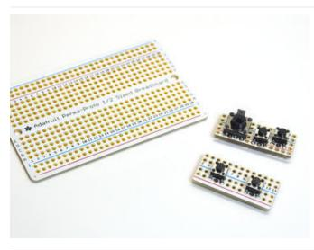
Perma-Proto boards are the bee's knees! They can be cut to size on a scroll saw, then the edges cleaned up and trimmed to a more precise size on a disc sander.
