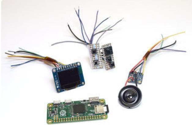
As a “farting around” project, the wiring, like the case design, wasn’t carefully plotted beforehand. All the wires were initially cut to a uniform 4" length and one end soldered to components, which were then moved around and each wire trimmed to a suitable length with a few millimeters slack, plus some extra to strip and tin.
