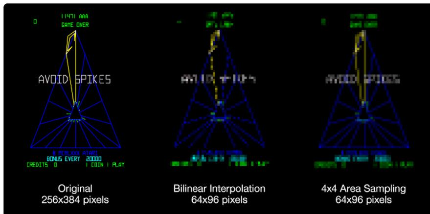
This software-based scaling isn’t the most optimal route...I’m certain Dispmanx could handle it on the GPU using a 2-stage bilinear scale with an intermediate canvas of some sort...but nanoscreen was just an evening project and I couldn’t get into that depth of understanding with Dispmanx; software scaling was familiar and comparatively easy, and runs well enough for what it is.
