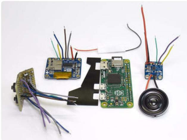
Making matters more challenging was the discovery that I only had two colors of 26-gauge silicone-coated stranded wire on-hand. That’s no help...26 gauge is too fat for this cramped space, and more colors really do help for keeping track of things, and better match the photos to the wiring diagram. So I made do with some inferior 28-gauge non-silicone wire, using the thicker stuff for just the few power-related connections. The process required patience, tweezers and a good soldering iron.
