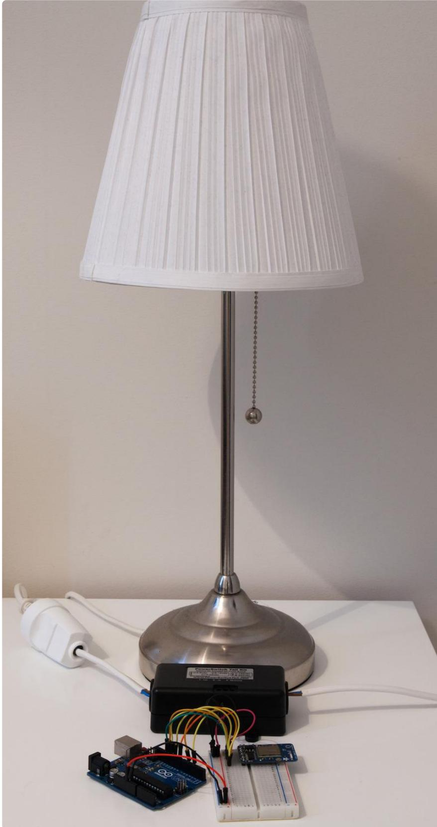
In this project, we are going to build an open-source version of WiFi power switches that you can buy in many stores. These switches can usually be controlled from a
