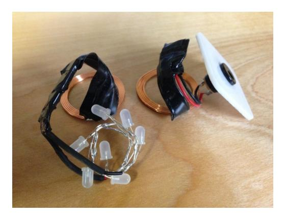
As you can see in the image above, I wired up the LEDs in parallel, then wrapped everything up in a healthy amount of electrical tape as best as I could to prevent a short circuit. The white piece of plastic was cut on a laser cutter to fit into my enclosure. There are plenty of ways you could make a nice enclosure for this with items found around the house.
