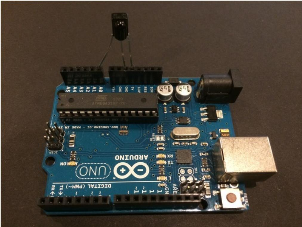
After loading the sketch from the Using and IR Sensor tutorial and making the two line changes suggested above, open the Serial Monitor from your Arduino IDE and press the blue Duo Pop Popper. The first part of your screen should look like below.
