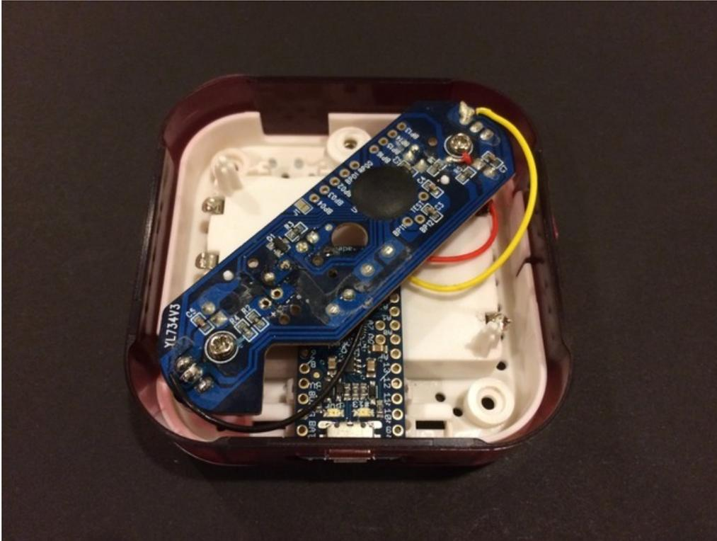
**Step 5:** Reassemble remaining portions of the case so you can program your newly built Duo Pop IR USB receiver module.
