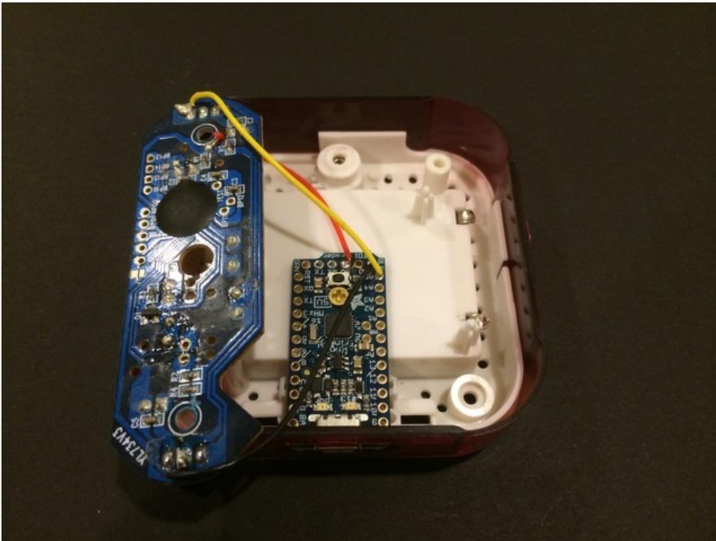
Step Four: Remount the IR module board to the case. Your IR to USB receiver should look similar to the picture below.
