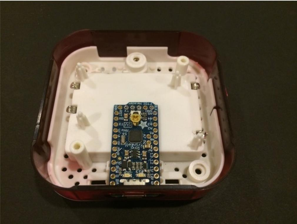
**Step Two:** Rewire and solder the IR sensor board wiring to the Pro Trinket as shown in image below. The only wire that remains connected to the original IR sensor board is the red wire. All other wires are removed, rearranged or resoldered to the original IR sensor board.
