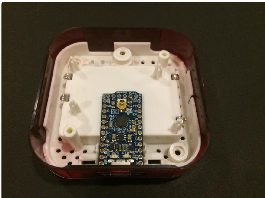
Step Two: Rewire and solder the IR sensor board wiring to the Pro Trinket as shown in image below. The only wire that remains connected to the original IR sensor board
