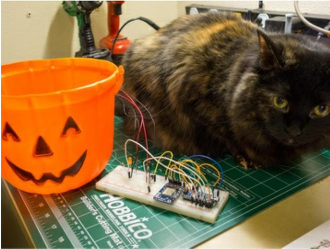
and LED about 1/3 of the way up the side of the bowl. You can also see the electronics that I built using an Arduino Nano, and a transistor to control current through the IR LED--the transistor isn't really necessary so it can be ignored.
