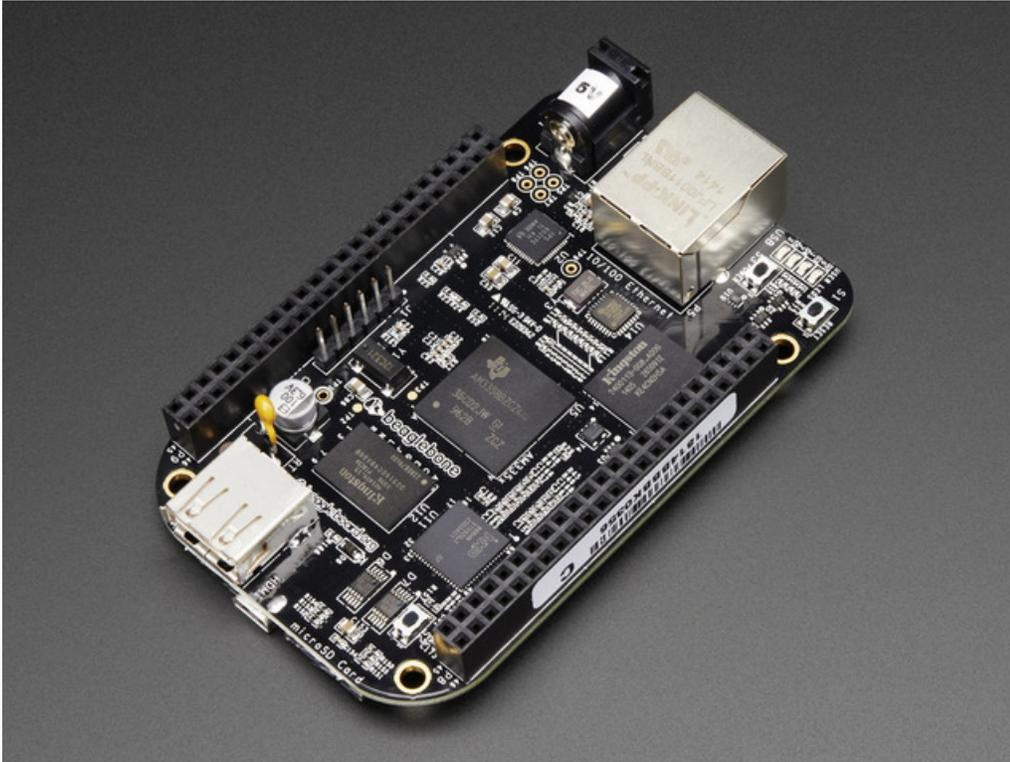
The **BeagleBone Black** is, like the Raspberry Pi, a little computer on one board. It features a substantially faster processor, onboard storage, and a broader array of hardware interfaces than the Pi. It also lets you connect to a nice web-based interface over a USB cable out of the box, which means you can get started without a spare keyboard & monitor or messing around with network configuration.
