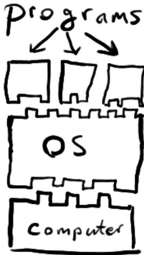
The kernel of a modern OS is a little bit like that `loop()` function, if you wrote it to enable all of the stuff that you might want to do with a general purpose computer. However, instead of just turning on/off an LED, it goes around to every single program and takes requests for what the program wants.
