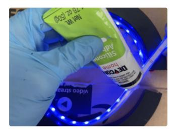
Next I glued the pixels in place around the inner edge of the frame, right at the bottom. The silicone coating on these pixels is tricky to glue -- very few glues will stick to silicone. My favorite is Devcon Silicone Glue (https://adafru.it/18Cn). It dries quickly, and clear-ish, and holds the silicone strip casing in place really well.
