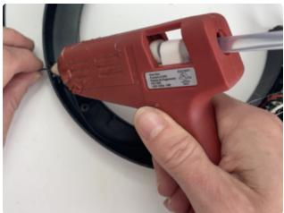
I plugged in the USB cable and fit my Pico W inside the frame, securing it with some hot glue. I threaded the USB cable through the channel at the back and glued that in place as well.
