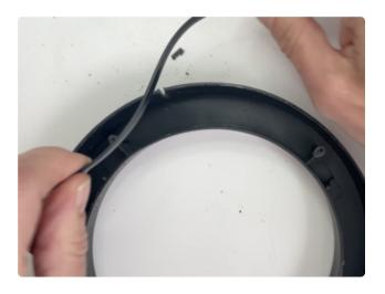
I plan to put the electronics inside the hollow frame, so I dremeled a channel at the back of the frame for my USB cable to pass.
