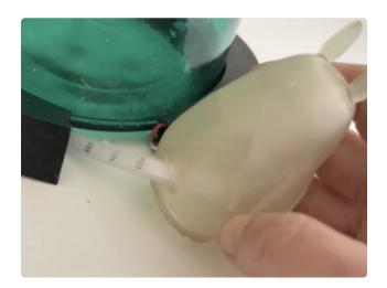
I drilled a hole in the back of Totoro and slipped in the last few LEDs from my NeoPixel strip. The clear resin clouded up just enough to diffuse the lights perfectly. Glowing Totoro, Hooray!
