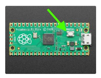
Start with your Pico unplugged from USB. Hold down the **BOOTSEL** button, and while continuing to hold it (don't let go!), plug the Pico into USB. **Continue to hold** the **BOOTSEL** button until the RPI-RP2 drive appears!
