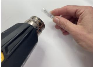
Once you're sure it's working correctly, seal up both ends of your NeoPixel strip by sliding the heat shrink over the solder joints then filling the heat shrink with some hot glue. While the glue is still wet, use a heat gun to shrink the heat shrink. This will form a waterproof seal on your pixels that will keep any rain splashes out.
