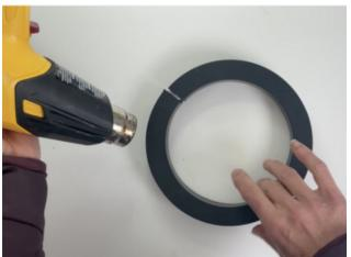
I removed the frame from the mirrored back, then cut through the side with a dremel. Then I heated the plastic frame gently with a heat gun until the whole thing was a bit soft and pliable, but not so much that it got melty.
