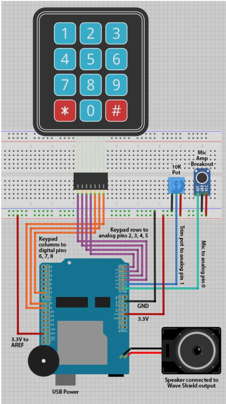
Upload the Adavoice sketch to the Arduino if you haven't already done this. If everything is wired up and loaded correctly, you should head a startup chime when the sketch starts (if using an SD card with the sample WAVs). If there's no sound, use the Arduino serial monitor and watch for diagnostic messages.
