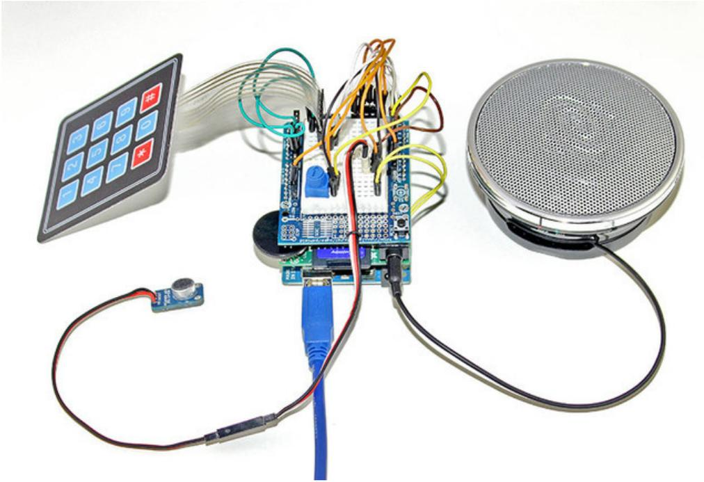
Once up and running, you can then talk into the microphone and should hear the altered result through the speaker or headphones (keep the mic away from the speaker to avoid feedback). Pressing any of the keypad buttons will stop the voice effect to play the corresponding sound, then resume afterward.
