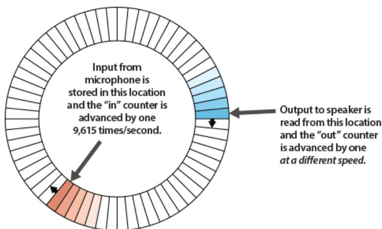
The frequency of recorded sound will seldom match the buffer length exactly, and audio samples are stored and read at different rates. This can produce a sharp discontinuity — a popping noise — each time the "in" and "out" points cross. A small extra buffer is used to store some of the prior audio samples, and the code cross-fades the audio over this boundary to reduce the "pop."
