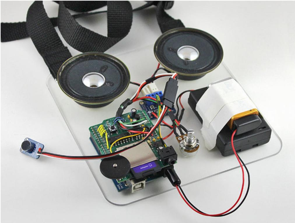
You can run the microphone connection a couple feet to reach inside a mask or helmet. A [servo extension cable](http://adafruit.it/973) (<http://adafruit.it/973>) provides a very handy 3-conductor separation point, so you can pop your head and set it down! Cut the servo cable in half, soldering one end to the mic amp board and the other side to the Arduino circuit.
