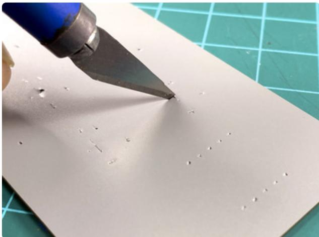
Slice holes through the vinyl for each component lead & use cross-cuts for the larger openings (switch posts, standoffs, etc)
