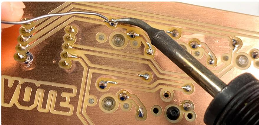
Solder both of the switch's pins to the bottom side of the PCB.
