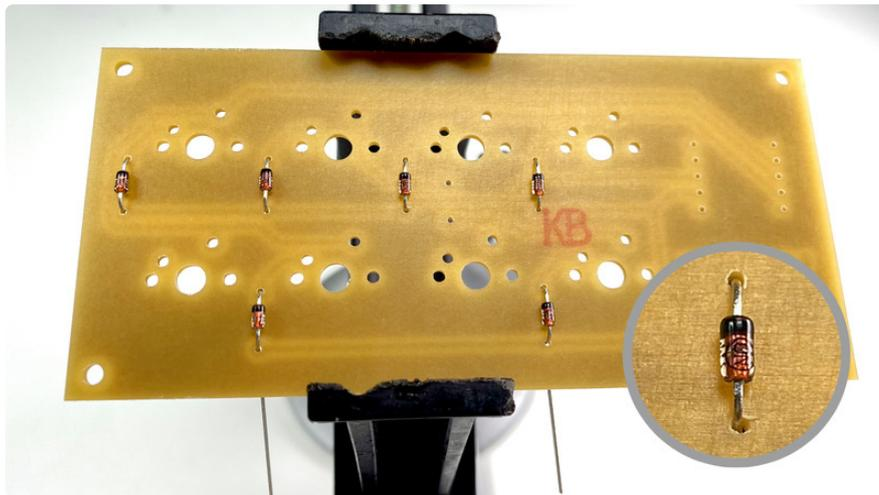
Mount the diodes on the PCB with each diode's **stripe** pointing toward the **upper edge** of the board as seen in the photo above.
