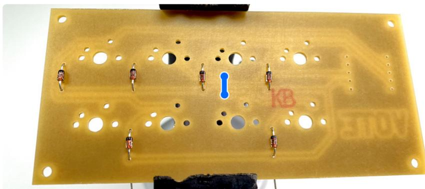
If you're working with a single-sided PCB, you'll need to install a **single jumper wire** in the location shown above in blue.
