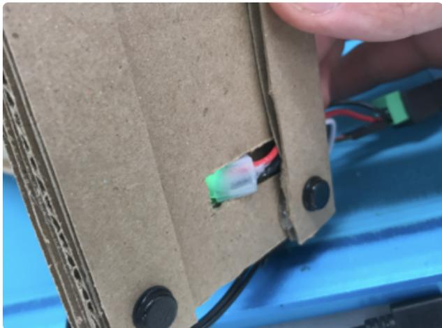
Add two more strips of cardboard to the bottom of the base, pinning the end of the NeoPixel strip so that it comes out the back.
