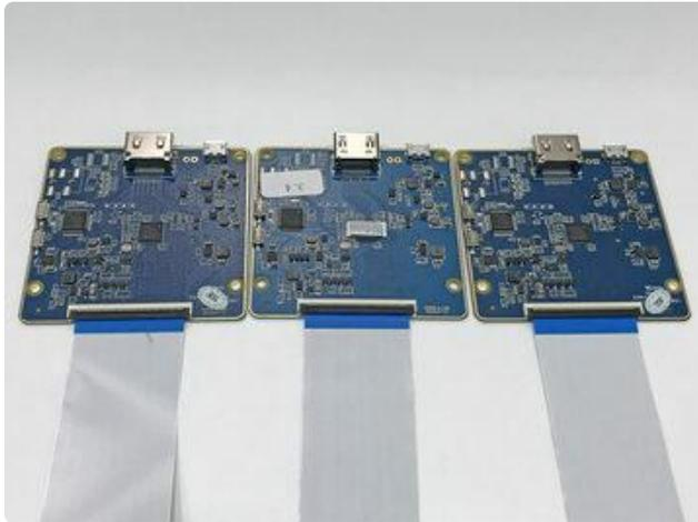
These displays must be paired with an HDMI adapter/driver board - they are not SPI devices. When buying, you may see separate options for a bare display (or two) and display-plus-HDMI-adapter for a bit extra, so make sure you get the latter.
