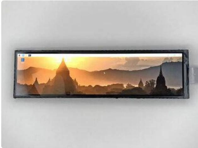
Originally for automotive use (backup cameras, rear view mirror, instrumentation) or rack-mount servers (system status). Many variants, from little-wider-than-16:9 to incredibly long and thin ribbons. Some include touch input, though there may be no software support on the Pi, depending on implementation.
