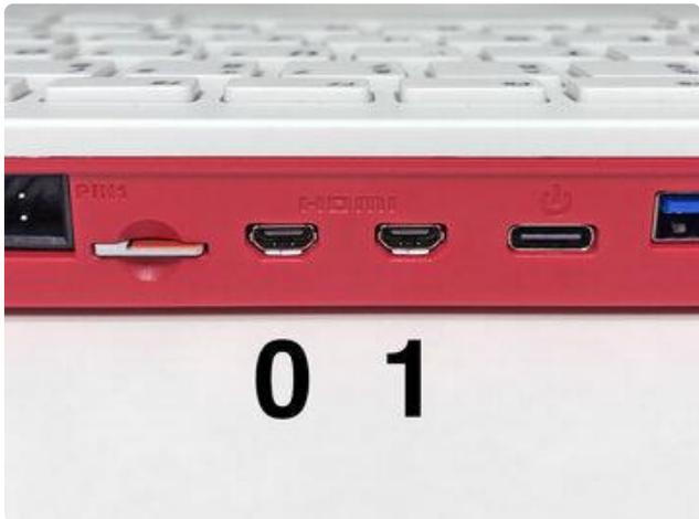
On the Pi 400, HDMI 0 is closer to the SD card slot, HDMI 1 is closer to USB-C.
