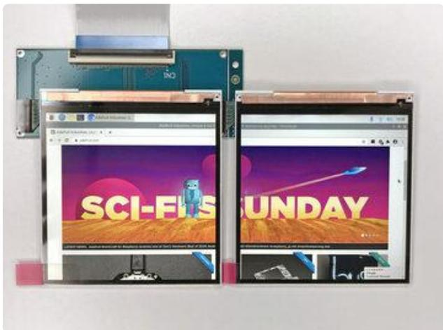
With a high pixel density for their size, and driven in pairs, these are likely intended for virtual reality headsets.
