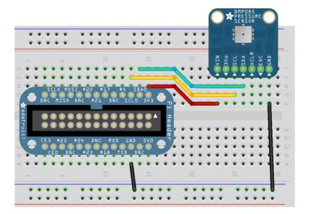
Make sure that you connect the VIN pin on the BMP sensor to 3V3, NOT 5V0! Connecting VIN to the 5V supply will cause the board to use 5V logic, which is perfect for the Arduino, but may damage the sensitive 3.3V inputs on the Raspberry Pi.
