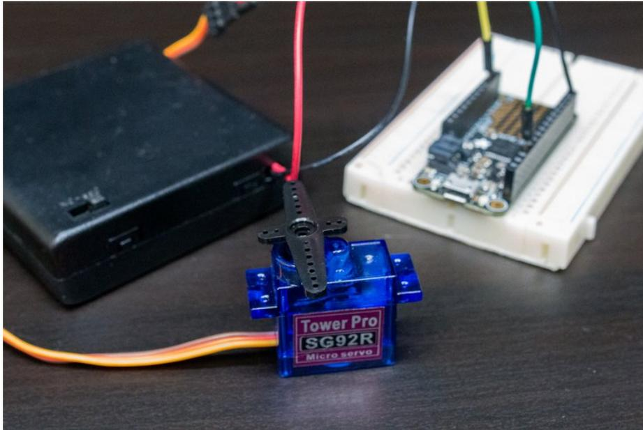
Servos are tiny motors that you can control the position of by generating a special signal. You might use a servo to move something back and forth, like moving a dial to indicate a measurement or even moving a latch to open and close a door. There are even special 'continuous rotation' servos that can act like little motors with control over their speed and direction—perfect for building a simple robot! The possibilities for movement with servos are unlimited!
