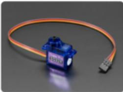
Set Servo Pin to D14, and keep the frequency at 50Hz.
