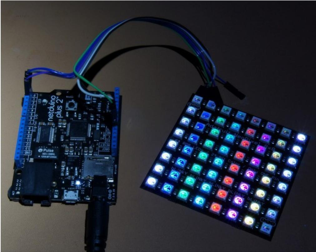
Even though there is lots of example code for NeoPixels for AVR, Propeller and PIC chips, it's a bit of challenge getting these LEDs to work with the Netduino. With the default firmware of the Netduino (any variation, Plus or no), it is not possible to send data to NeoPixels.
