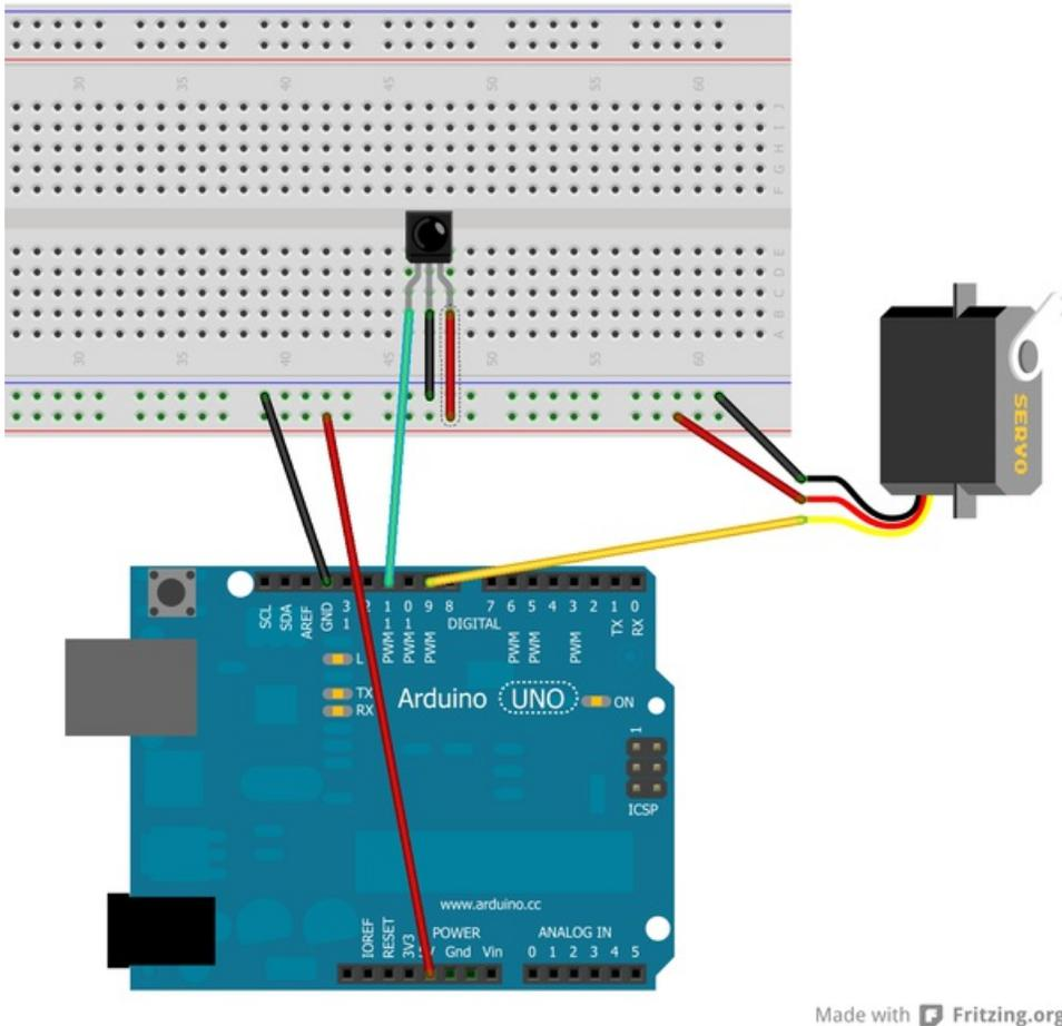
NOTE: The above illustration shows the receiver on pin 11 however the sample code uses pin 2. Any digital input pin can be used.
