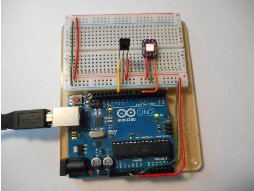
In this very simple example we will change the color of a NeoPixel by pushing buttons on the remote. We are using a single pixel but you can modify the sketch to control an entire strip or matrix. For more information on NeoPixels [visit this guide in the Adafruit Learning System \(https://adafru.it/dhw\)](https://adafru.it/dhw). Here is the code:
