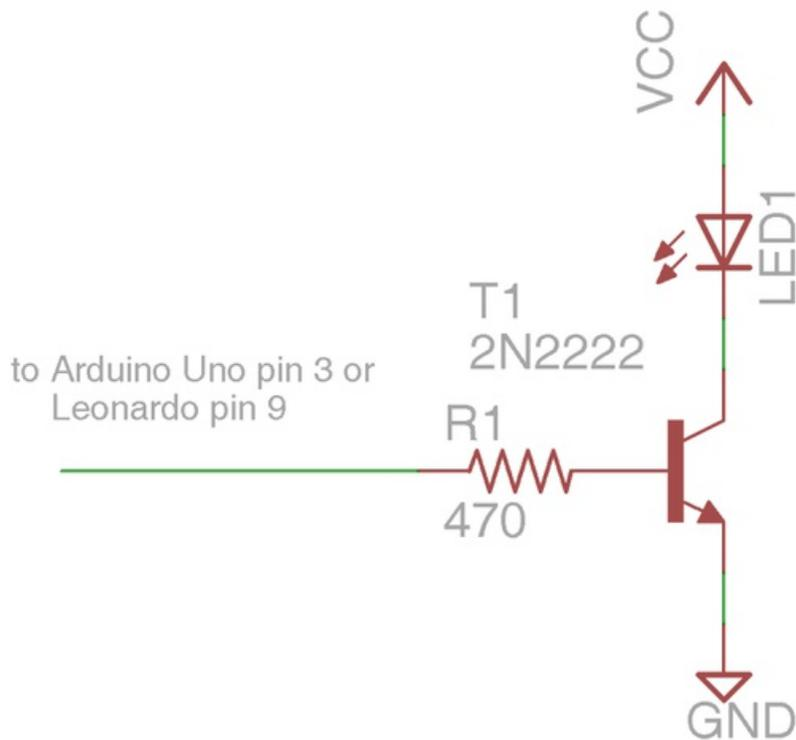
Make sure that you get the polarity of the LED correct. The shorter of the two leads connects to the transistor and the longer one connects to the positive supply. Note that the current passing through the LED will in all likelihood will exceed the maximum continuous current rating. However because the signal is modulated and sending a sequence of pulses that will only last a few milliseconds the circuit will work fine.
