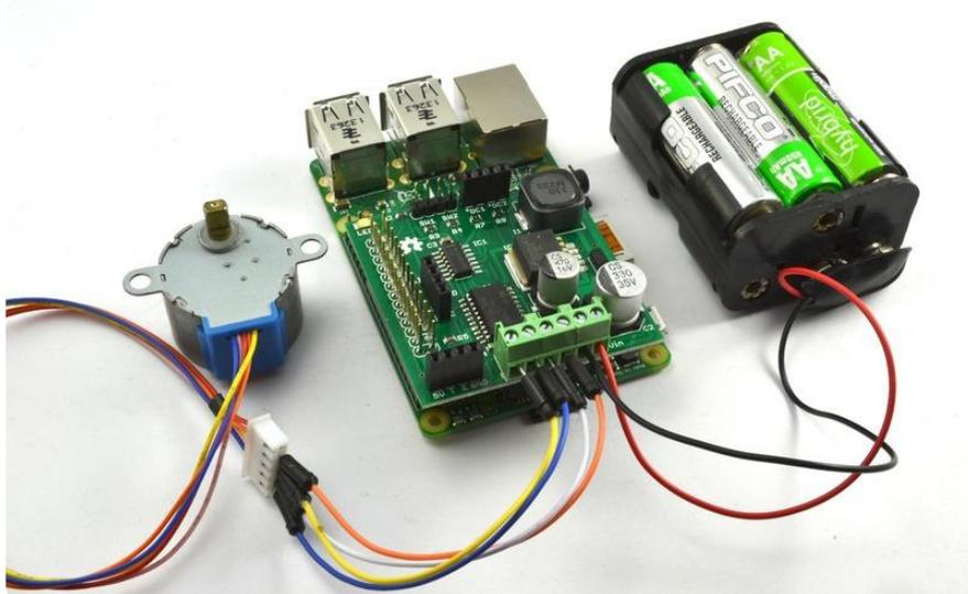
Note that the RRBv2 is not suitable for use with 12V stepper motors.
