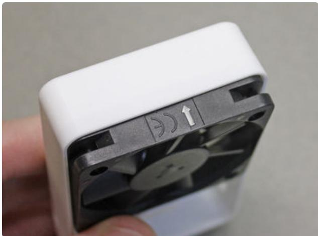
Check the fan's airflow direction arrow, make sure it's pointing front to back. We're installing in the back of the case.
