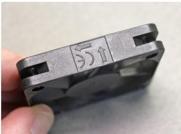
Check the sides of the fan...on one face should be an arrow indicating the airflow direction. Confirm that the fan is in fact blowing in this direction...if not, you may have the + and – wires reversed.
