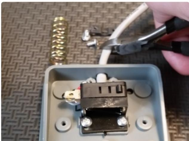
Using wire cutters, cut the cable about 1.5 inches (4 centimeters) past the pedal base.
