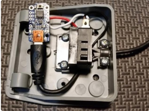
If you have not done so, strip 3/8" (3 millimeters) of insulation from the red and white wires. Solder the white wire to the GND pin on the Trinket. Solder the red wire to the #0 pin on Trinket.
