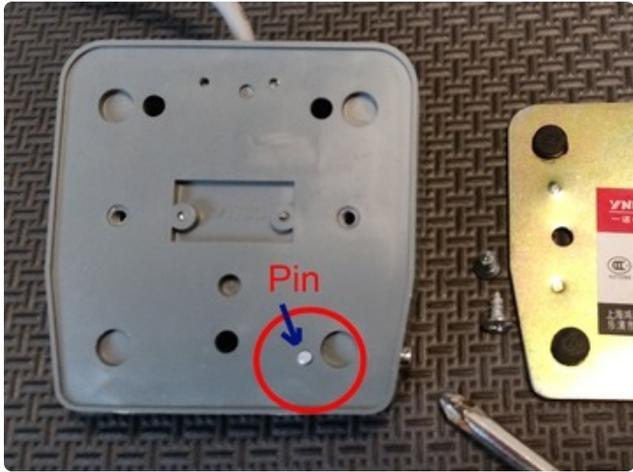
Turn the pedal over and using a medium Phillips screwdriver, carefully remove the metal back cover.
