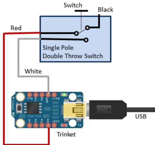
The wiring is shown above. The existing foot switch wires are cut short and two connected to Trinket pins #0 and GND (ground). When the foot switch is activated, the switch contact pair that creates a short connects Pin #0 with ground. When the Trinket detects the pin connected to ground, it outputs one or more characters as a PC keyboard.
