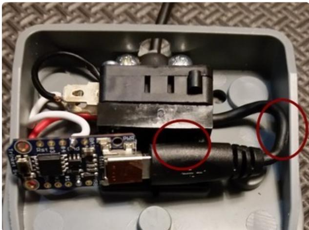
Tuck the Trinket and the cable up next to the switch. The top of the trinket board should not protrude above the switch so it will need to be placed at a slight angle.
