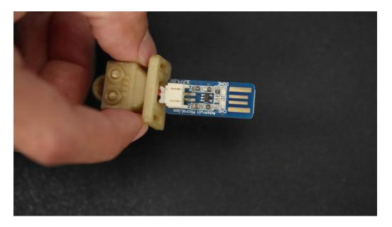
Connect the Micro Lipo USB charger to the female JST Port. Make sure the orientation matches the photo above.
