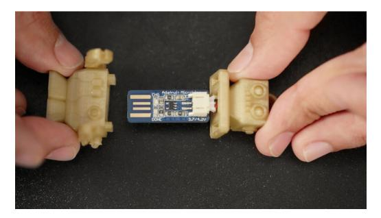
The Micro Lipo USB charger should be inserted to the **lipobot-body.stl** part with the gold plated usb port facing the orientation of the robot. Slide into place and apply a bit of force to the **lipobot-head.stl** part so it clicks into the **lipobot-body.stl** part. It may be a bit hard, but the tolerances will loosen a bit over a couple of uses.
