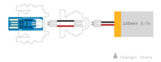
A short JST cable fits inside the cavity of the head cap with the female connector accessible from the back of the cap. The male connector extends out through the bottom of the cap and connects to the Micro Lipo USB Charger.
