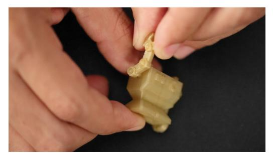
Loosen the holes on the two arms and the body with an x-acto knife. Test fit the pins into the holes by turning them until they can fit all the way through the holes. Insert the pins through the arm parts and into the body. Press the two pins all the way through, you should be able to freely rotate them.
