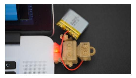
Plug in a lithium polymer battery and watch it charge! The little grabbers on the arms can optionally hold onto the JST cable.
