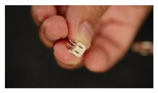
Bend the two terminals from the end of the JST connect so they protrude straight out. Tin the terminals and solder them to the ground and positive wires of the JST cable. Use heat shrink tubing to secure the connections.
