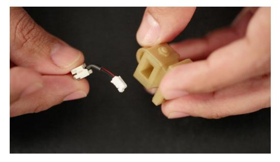
Test Fit JST Cable Insert the shortened JST cable into the **lipobot-head.stl** part with the male JST port first.
