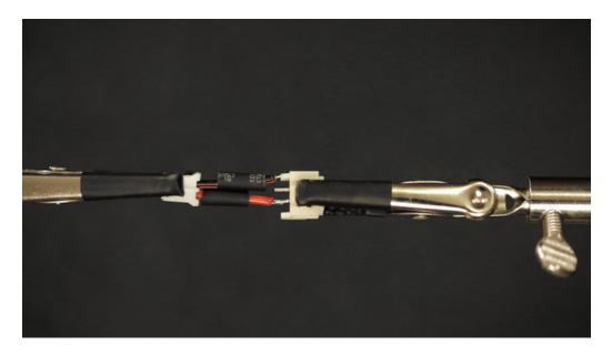
Use a third-helping hand to assist you in soldering the JST cable to the JST connector. Solder the tinned ends of the ground and positive wires of the shortened JST cable.
