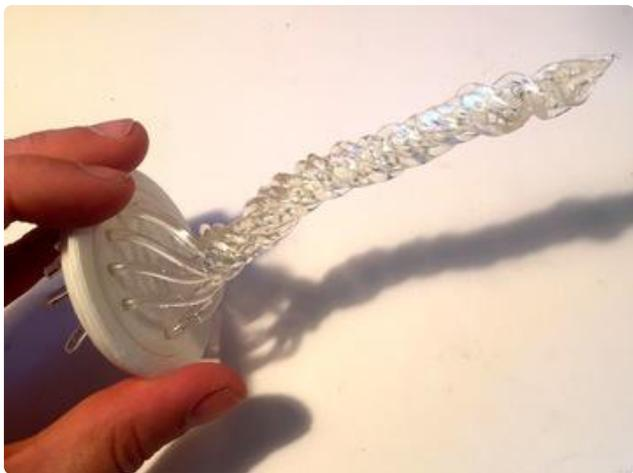
To finish it off at the top, I trimmed each piece of light pipe slightly longer than the last in a spiral, and carefully melted them together. I left the very last piece extra long, then melted it with the heat gun and pulled, stretching it into a perfect point.
