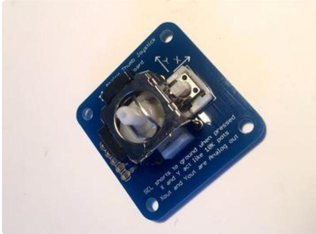
Place the joystick on top of the breakout board -- it only fits one way.
