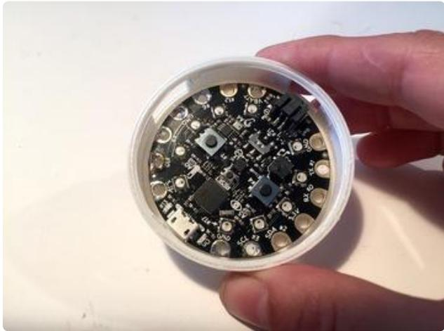
Temporarily attach the cover to the lid ring. Put your Circuit Playground inside the base, and screw the lid on.
