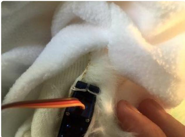
Once you're happy with placement, sew and/or glue the servo in place on the hat, hiding it inside the fabric. Don't sew the EAR in place -- it should be free to move! Just attach the servo.
