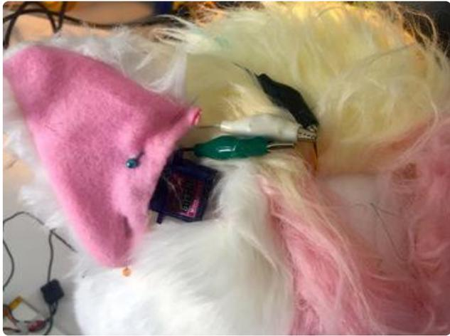
Attach some alligator clips to the three wires and hook them up to the Circuit Playground. Move the ear back and forth with the joystick and play around with proper placement on your hat. I ended up adding another little stitch to make my ears flop over a bit more.
