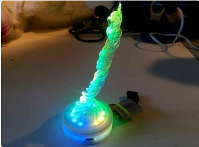
Use a sharp pair of scissors or snips to trim the underside of the light pipes to 3mm, so they just touch the neopixels when the Circuit Playground is encased in its 3d housing.
