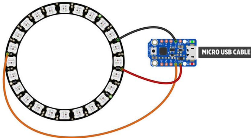
Follow the diagram above to connect the NeoPixel Ring to the Trinket. You can measure the wire lengths by mounting the ring and Trinket to the 3d part and then cutting the required sizes for each pin.
