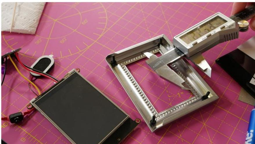
Once the spot is marked, take a Dremel or similar tool and carefully drill out a hole for the light sensor to be exposed. You'll want to make it slightly bigger than the sensor so that you won't get any unnecessary shadows that will affect the code.
