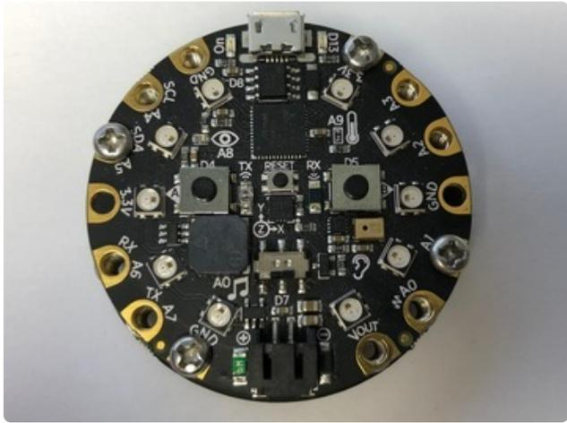
Install a few screws loosely, so that all of the holes are still aligned, before tightening them down.
