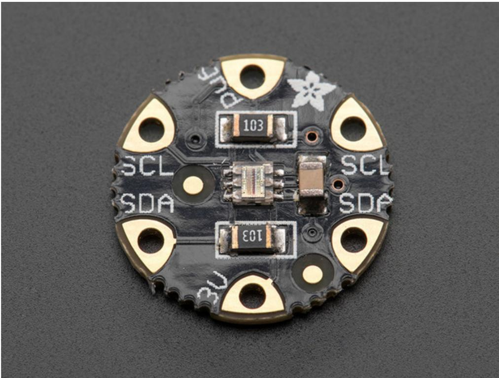
The sensor has a digital (i2c) interface. You can select one of three addresses so you can have up to three sensors on one board - each with a different i2c address. The built in ADC means you can use this with any microcontroller, even if it doesn't have analog inputs. The current draw is extremely low, so its great for low power data-logging systems. about 0.5mA when actively sensing, and less than 15 uA when in powerdown mode.
