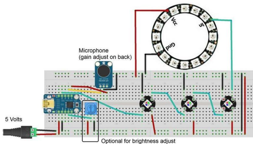
The best way to start is to breadboard first. You can then transfer the circuit to a small perma-proto board when you are satisfied with your circuit and want to consider a permanent mount.
