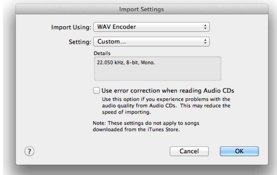
For voice recordings, 8 KHz is often a sufficient sample rate. For music, 16 KHz or more. Generally, higher sampling rates will produce better-sounding audio, but it requires more space. Also, the way the playback circuit works, there's diminishing returns above 25 KHz. Experiment!
