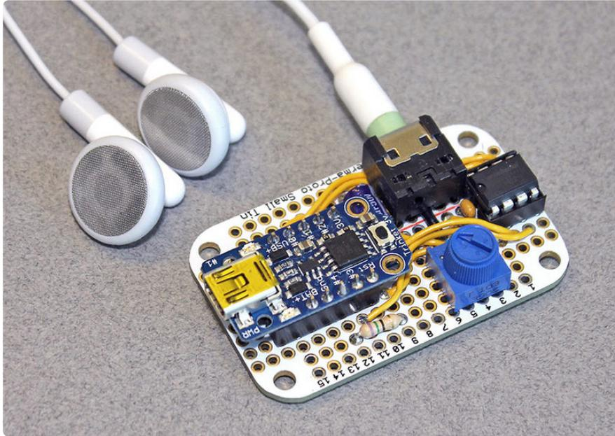
We usually think of the Adafruit Trinket as a tiny subset of a “real” Arduino; less RAM, less code space, less I/O. But this little chip has a couple tricks up its sleeve, things its larger brethren can’t do. One of these is a high-speed PWM mode. With just a few extra components this can be used for audio output. Not simply piezo beeps and buzzes...actual sampled digital sound!
