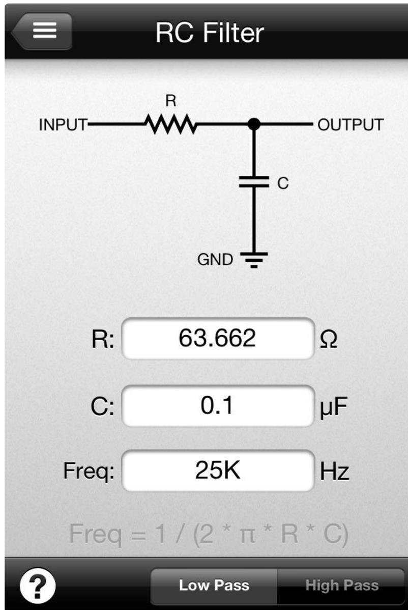
For a 25 KHz cutoff and 0.1 microfarad cap, the calculator suggests a 63 Ohm resistor. That's not a standard value you'll find anywhere, so we just select the next common size up from there: **68 Ohms**. I happened to have a bunch of 75 Ohm resistors around...that's close enough, this isn't precision work.
