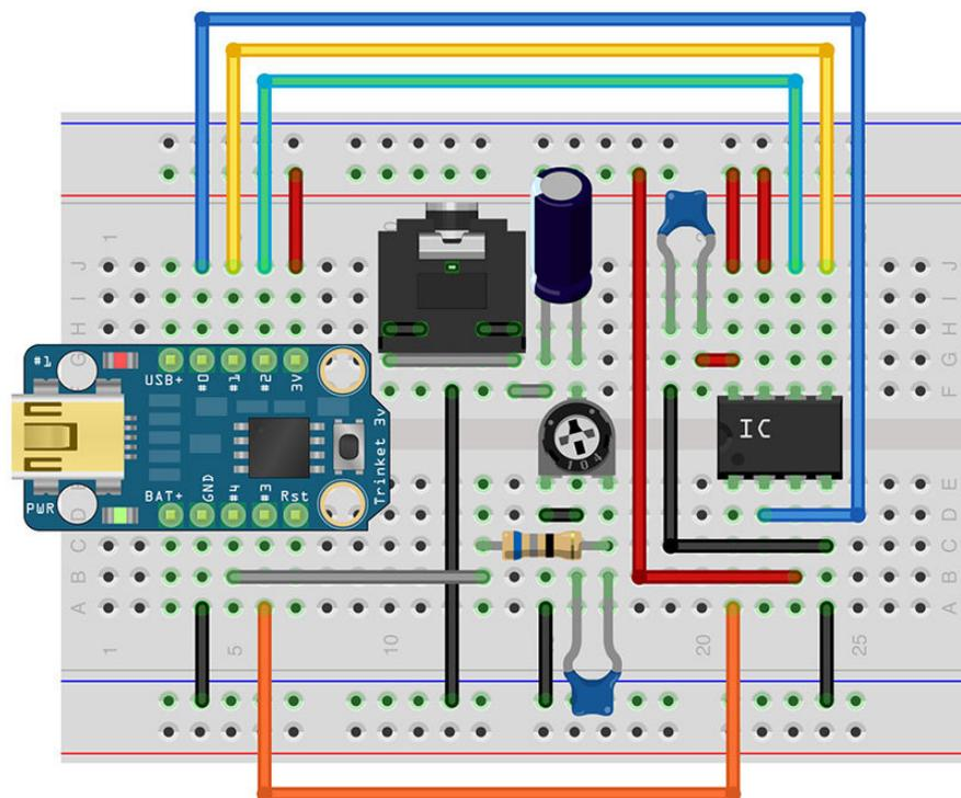
The power source can be anything the Trinket can handle: a small 3.7V LiPo cell, three or four AA or AAA alkaline cells, etc. You can also plug into USB, but there's a 10 second timeout while the bootloader runs its course before the playback sketch runs.
