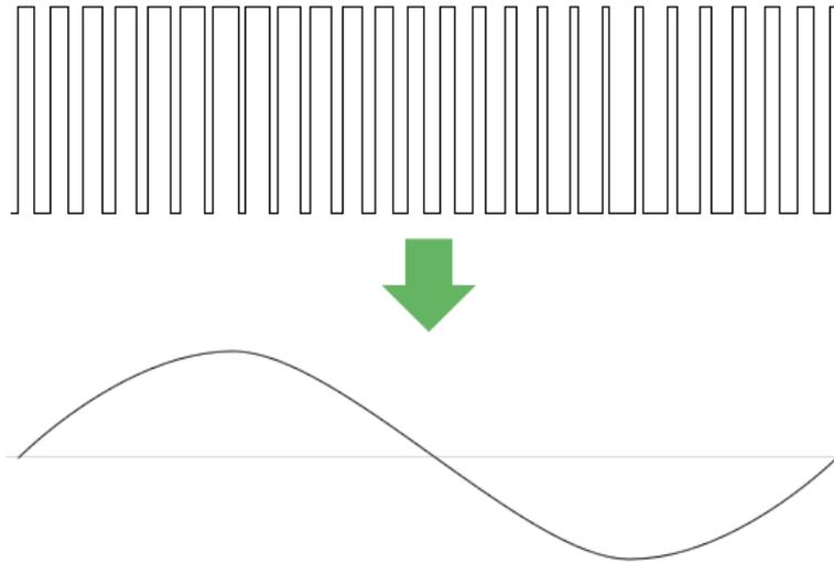
A very basic low pass filter can be made from just a capacitor and resistor. First we need to know the filter's cutoff frequency — frequencies below this pass through, while higher frequencies (like the PWM signal) are attenuated. A rule of thumb with PWM audio is that the highest usable audio frequency (our cutoff frequency) is about 1/10 the PWM rate. The latter we've already established is 250 KHz, so a good cutoff would be 25 KHz.
