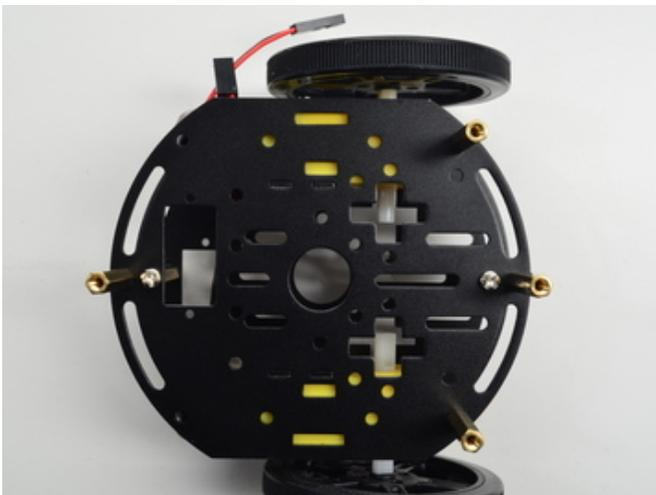
Screw the remaining 2 or 4 standoffs into the second chassis layer.
