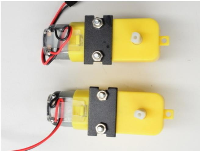
Screw the two black panels onto the motors. The metal panels go on the side with the red and black wires coming out
