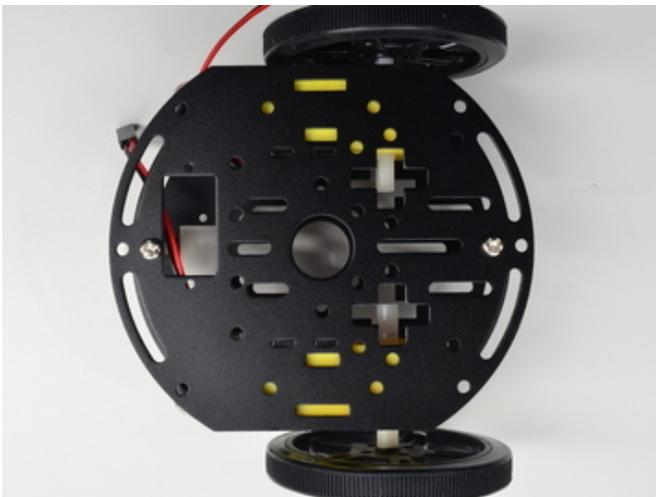
Place the next layer of the chassis on top of the motors. *In this photo we didn't line up the second plate just like the first plate (note the off-set rectangle cut out) - this might fit for you or you might have to line them up with the same cutout to get a good fit*
