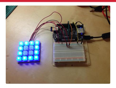
Adafruit Trellis (http://adafru.it/1616) is a great system for adding backlit keys to your own projects. Trellis' elastomer keypad acts as both an input and fully addressable LED display. You can even tile multiple Trellises together to form large, captivating displays.
