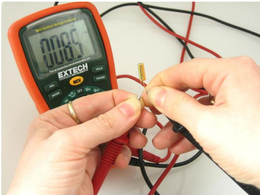
When pointing up, the switch is closed (low resistance / continuous).
