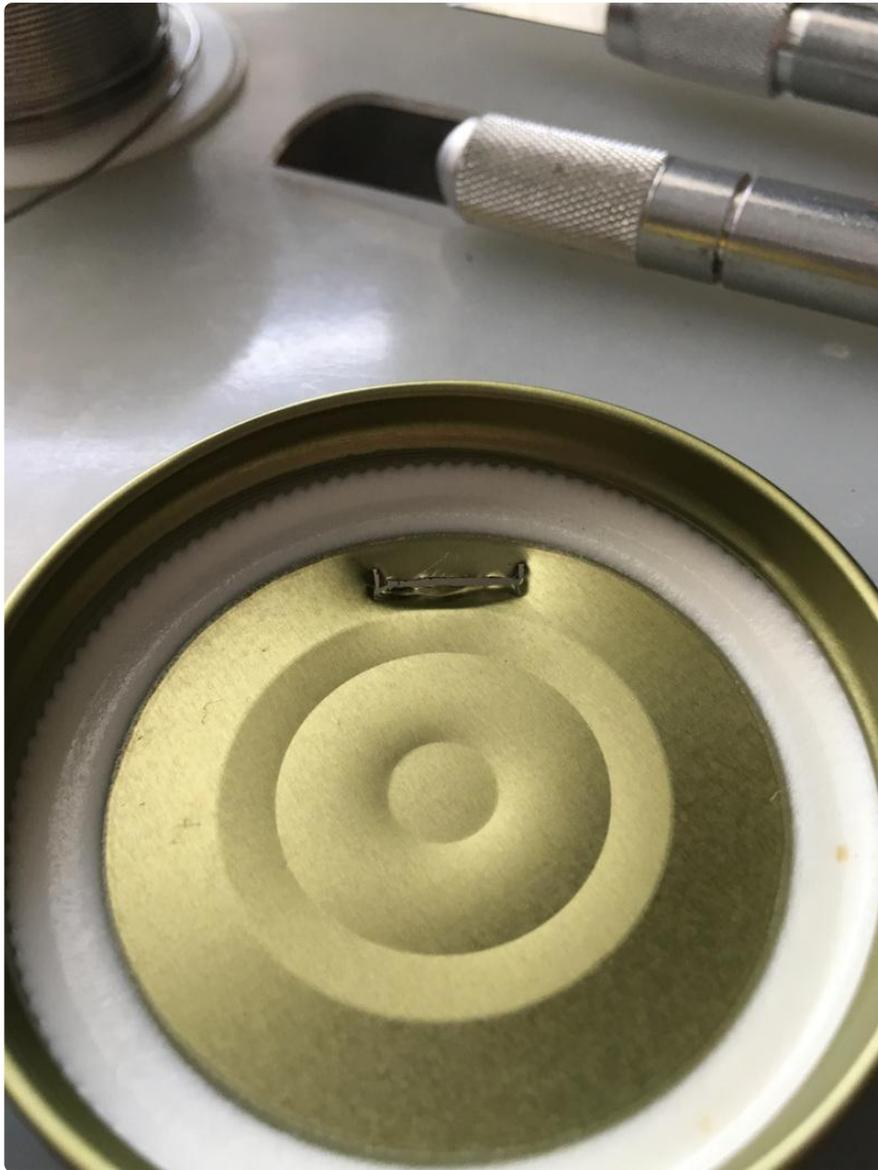
The sensor is placed inside the jar and, for my build, long headers are used to go through the lid of the jar to the electronics on top of the lid.
