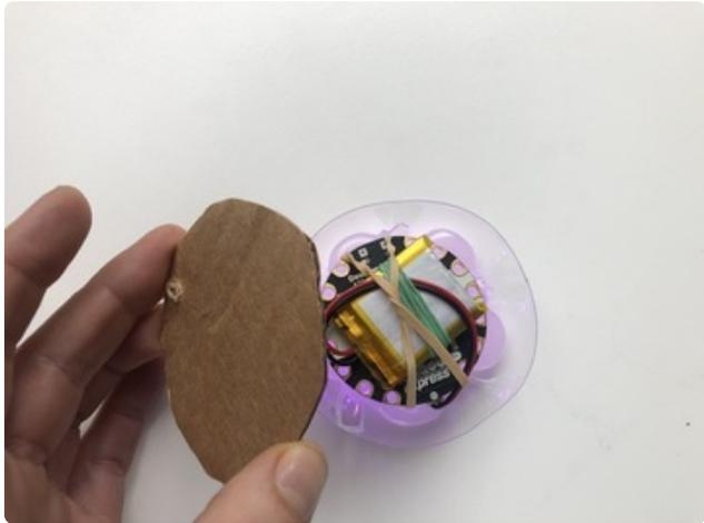
Place the Circuit Playground into the gem and place the back on. Use some scotch tape on the opposite side from the hole to hold it in place. Thread a necklace cord or string through the holes in the cardboard and the plastic. Now you have a wearable gem!
