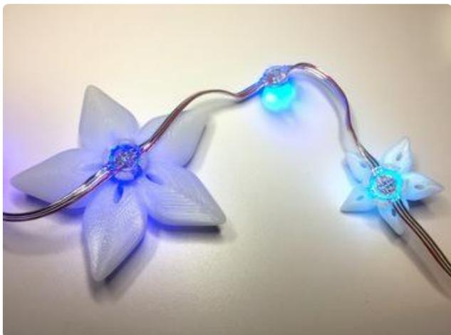
Clip the 3d printed flowers gently onto each light. If they don't seem to fit right, turn them 90 degrees -- the spacing between the clips is not exactly even; the wire goes between the wider clip spacing.
