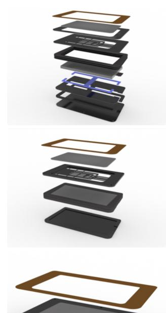
To show off the panel, I built a delicious frame/case sandwich to hold the backlit panel, LED matrices, and the electronics and wiring in place.
