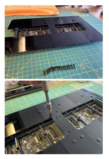
A second bracket layer is laid over the first and then they are both screwed to the LED panels using M3 screws as shown.
