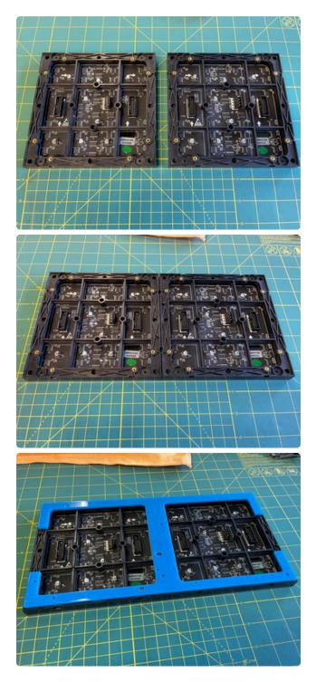
Matrix Bracket To hold the two LED matrices together, a custom bracket is used.
