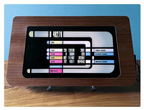
To use the display, plug in both the USB-C power and the 5V 4A power. The display will start up automatically.
