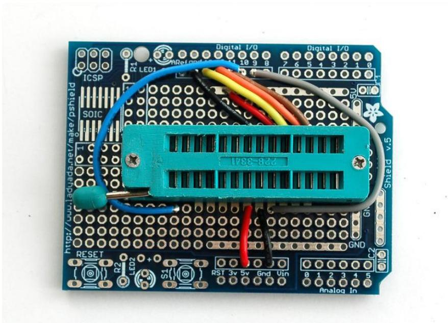
Follow the protoshield tutorial to solder in the Red LED into LED1 position, Green LED into LED2 position. Also solder in the two 1.0K resistors next to the LEDs. We'll use the LEDs as indicators. Then solder a wire from the LED2 breakout (white) to analog 0 and a wire from LED1 breakout (white) to digital 8.
