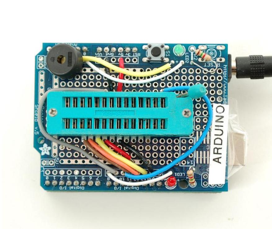
Finally, you'll need to solder on the header to allow the shield to be placed on, break the 0.1" male header and place it into the Arduino sockets. Then place the shield above on top to solder it in place.
