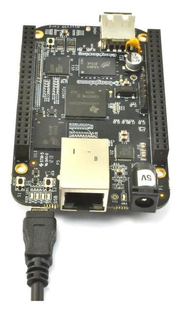
This lead can server the dual purpose of both supplying power to the BBB and allowing the BBB to emulate a USB modem. It is this trick that allows the BBB to be accessed as if it were networked, allowing you to communicate with it using a browser or SSH client on your computer.
