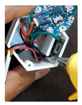
8) At this point, the soldering is complete. Lets program the Gemma before final assembly. You will need the <u>Adafruit NeoPixel library</u> () for the sketch. Grab the <u>Arduin o sketch</u> () and load it onto the Gemma. Putting the Gemma into the bootloader mode is documented here ().
