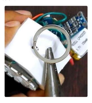
11) Lets do the final assembly by inserting the battery first, then the Gemma.
