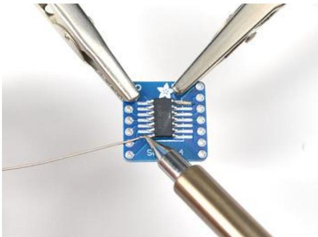
Now you can 'fix' the chip in place by soldering in the opposite corner. The one pin you soldered will keep the chip in place mostly, so you just have to solder the other pin a little to make the setup secure
