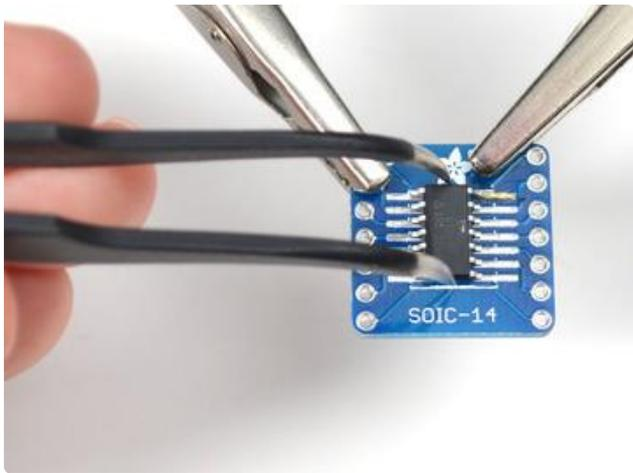
Once you've identified which is pin 1, hold the chip with the tweezers over the pads and then re-heat the corner pad you soldered onto a few steps ago.
