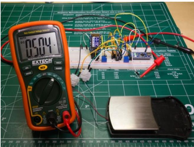
Adjust the output offset trim potentiometer with no weight on the scale until the output voltage is around 0.5 volts.
