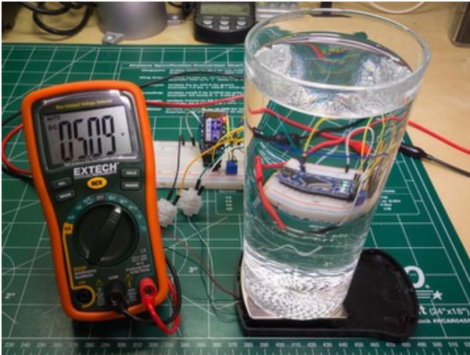
Adjust the gain trim potentiometer with a full glass of water on the scale until the output voltage is around 5 volts.
