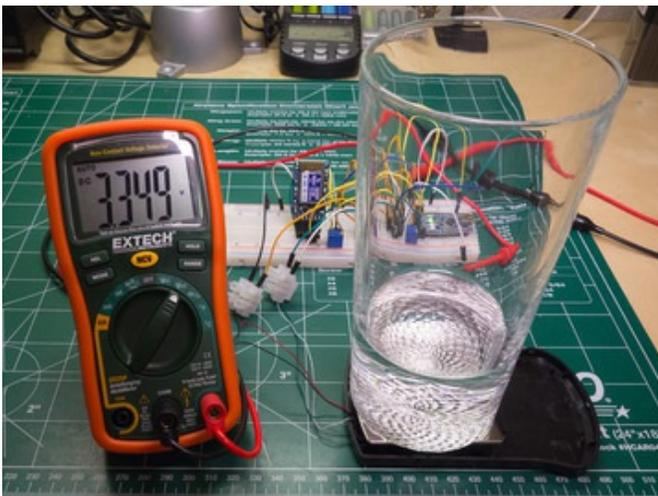
Check that when some weight is removed from the scale, the voltage drops to a value between 0.5 and 5 volts. The voltage on the output of the amplifier will be proportional to the weight on the scale.
