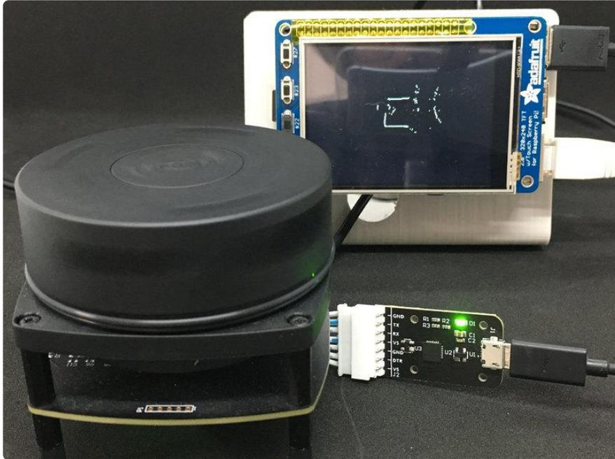
LIDAR is all the range\*. It's one of the fundamental sensing technologies of autonomous vehicles. It gives a system the ability to see how far away things are 360 degrees around it.
