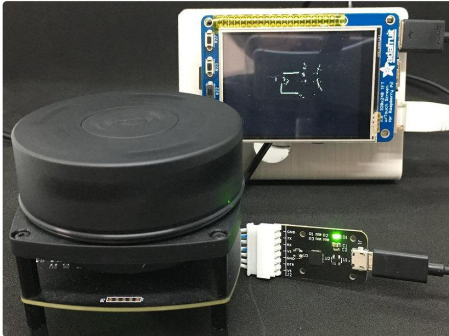
The simplest way to use the RPLIDAR with a Raspberry Pi is to interface through the bundled USB adapter. Connect a USB cable on the Raspberry Pi and then plug the other end into the LIDAR USB adapter board. Ensure the adapter board is fitted correctly onto the sensor per the instructions in the manual.
