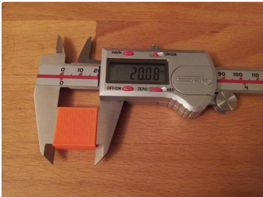
Scale calibration illustrates the process in which you compare the desired dimensions with the actual dimensions your printer produces. The easiest method for accomplishing this is to start by printing a calibration object, like a [Calibration Cube \(\)](#) or the [Calibration Vector \(\)](#). Once complete, use a set of calipers to check the dimensions and record your results.
