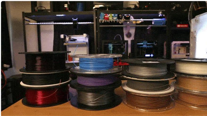
Although there is a wide range of filament types a 3D printer can handle, ABS and PLA plastics are by far the most popular. These two plastics are readily available in a staggering amount of colors, even glow-in-the-dark!
