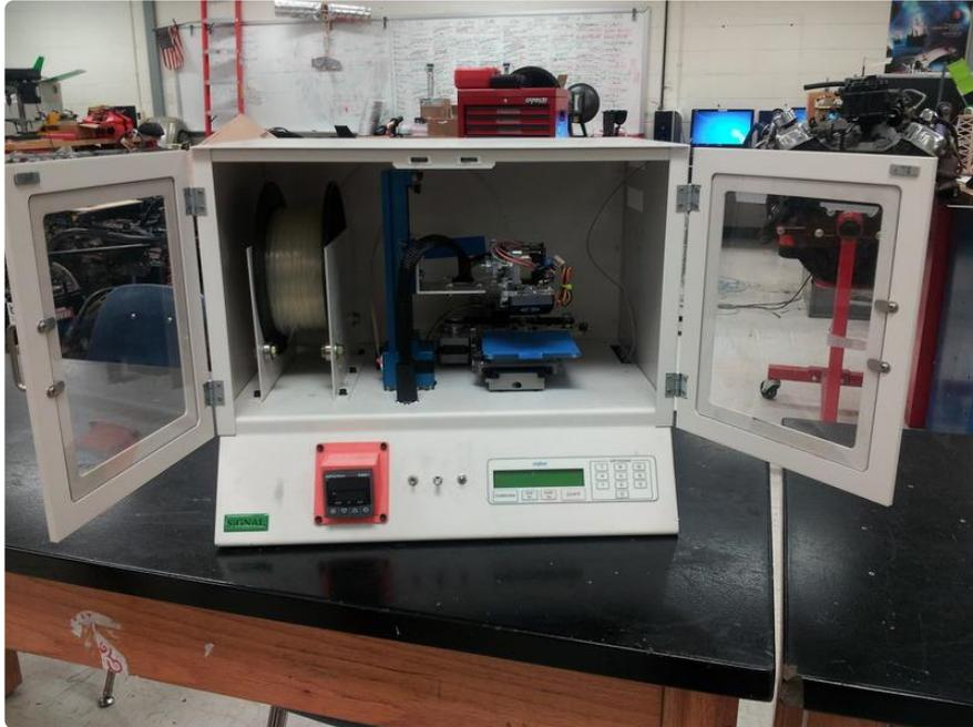
The 3D printer uses a process called fused deposition modeling to construct a solid object from a virtual model. This process involves the controlled deposition of a molten feed stock, typically ABS or PLA plastic, onto a build surface where layer-by-layer the model emerges. Each 3D printer features a series of motors to move the three axis and the extruder, and a controller to move the motors and manage the build process.
