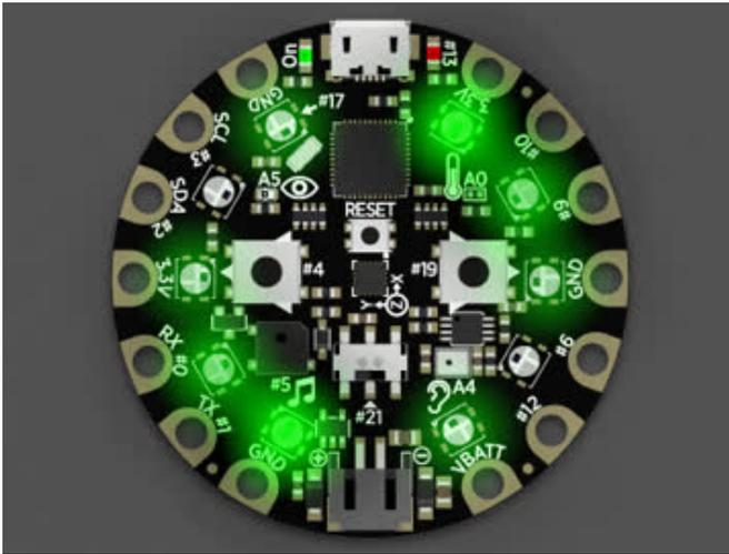
Tapping again switches to this sine wave spinner. Rather than on-or-off, the brightness of each pixel is determined by a moving sine wave. *I really like effects like this, they give electronic projects a more “living” feel than the usual blippy animations. But I digress...*
