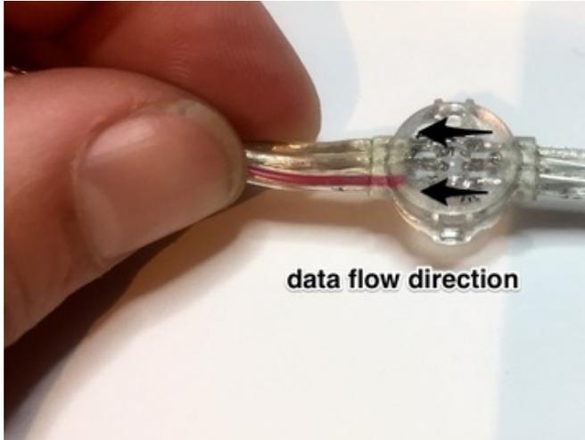
NeoPixel color data must travel from the “in” end of the strand to the “out” end. Examine the backs of the pixels *very* closely. Printed on the PCB, you might see either some data direction arrows, or the words “IN” and “OUT” between pads. The weatherproofing epoxy makes things murky and you may need to look at several pixels before finding one. This is important! If you connect the microcontroller to the wrong end, the lights won't work.
