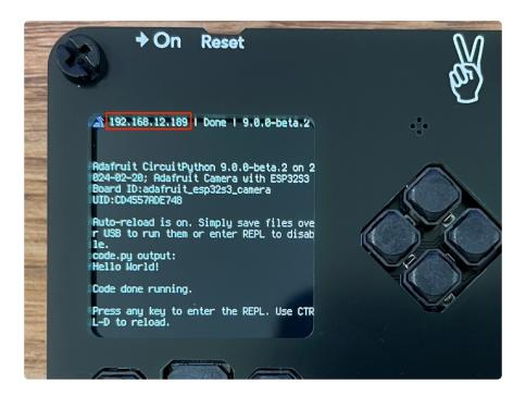
If it launches code instead of displaying the REPL, you can try connecting to the serial console with a terminal application. For more details on how to do this, you can take a look at the Connecting to the Serial Console (https://adafru.it/19FA) page.
