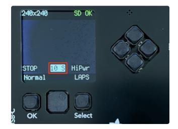
Now using the left/right buttons, select the time interval between photos and adjust to whatever you like. For the purposes of this example, it will be set to 10 seconds.
