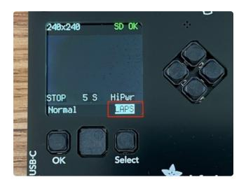
Press the **left/right** buttons, move the selector over to the mode option in the lower righthand side of the screen. It should say **JPEG** if you haven't already adjusted it. Once it is highlighted, use the **up/down** buttons to change it to **LAPS**.
