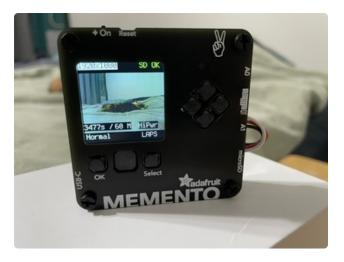
Set up your MEMENTO camera to point at the subject that you would like to take a timelapse of and press **OK** to start. You may wish to set the camera on a steady surface so that it doesn't inadvertently tip over while recording. The timer countdown will start and after it finishes, it will save a photo on the SD Card.
