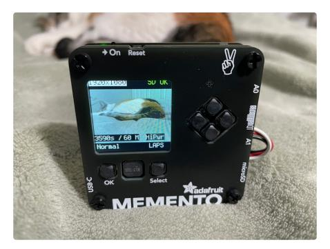
Web Workflow is an excellent way to update your MEMENTO camera board remotely. If your project involves keeping the MEMENTO in a specific position or perhaps it is mounted in a difficult to reach place, then editing your code with Web Workflow will be essential.
