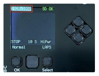
If desired, change the resolution to one for which you would like to capture images. The default is 240x240 pixels, but you may desire a little bit higher resolution than that.
