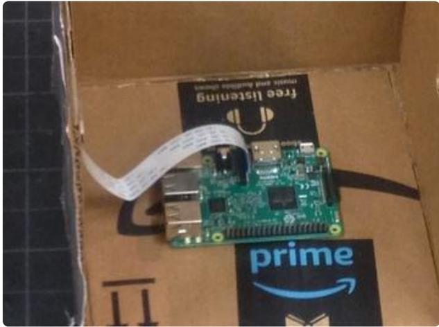
Glue the sides together to form a part of a cube. Connect the camera to the Pi.
