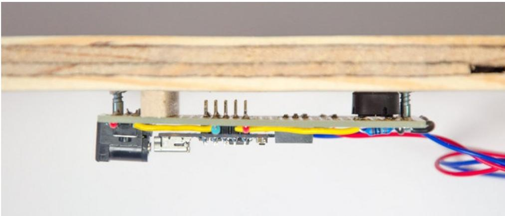
After everything is in place and tested, tack the cables in place with hot glue, cable ties, or cable staples.
