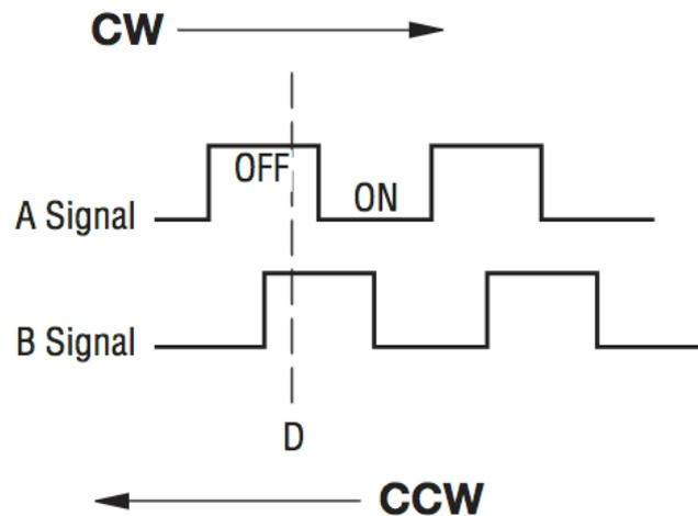
When rotating clockwise, the A pin connects first, followed by the B pin. When rotating counterclockwise, the B pin connects first, followed by the A pin. By tracking when each pin connects to and disconnects from ground, we can use the signal changes to determine which direction the knob is being rotated. The order in which they change is based on the direction the knob is being rotated. Tracking the signal changes allows us to use the rotary encoder as an incremental input.
